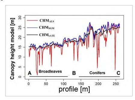
Figure 55 Vertical profile showing comparison of CHMs along the selected transect line
