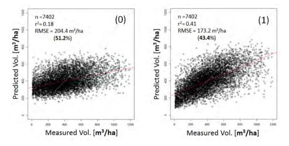
Figure 44 Goodness-of-fit plots where measured values are plotted against RF model predicted forest volume for model without (0) and with (1) TanDEM-X IDEM based canopy height information. The other input variables in both 0 and 1 remain the same.
