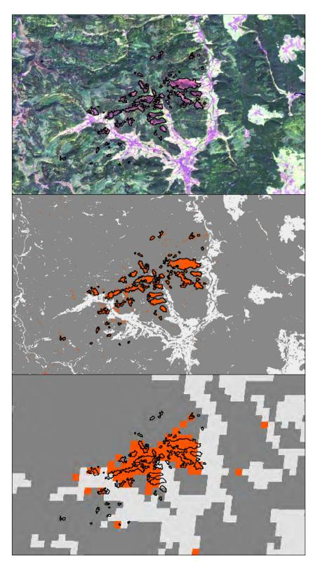
Figure 27 Assessment of storm damages in an area nearby Freiburg in Germany. Above, Landsat data with 30m spatial resolution overlaid with visually delineated storm damaged areas are shown. In the centre, a result of the landsat based assessment is drawn and below the results from low resolution MODIS assessment is shown.
