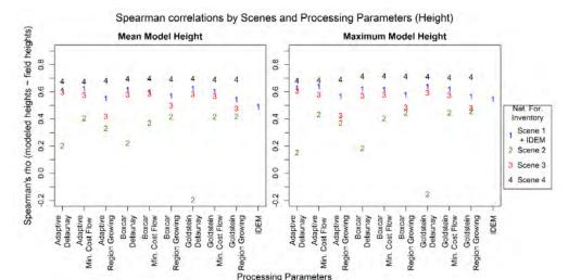
Figure 41 Spearman correlation coefficients for relationship between modelled forest heights and field heights by processing parameters, scenes and use of mean and maximum model height values. Processing Parameters: applied noise filter and phase unwrapping of the particular forest height model used for the analysis
