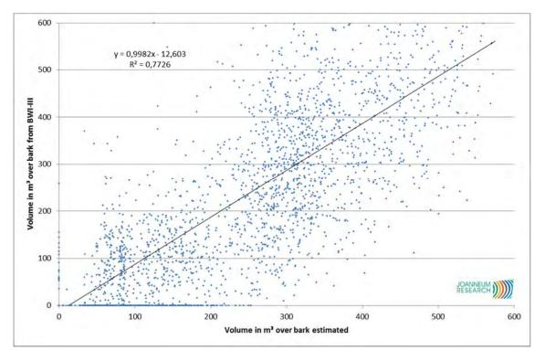
Figure 28 Independent accuracy assessment for estimation of stem volume. Scattergram and linear trendline based on n=5.167 sampling locations (each consisting of four NFI-plots) from the third national forest inventory of Germany.
