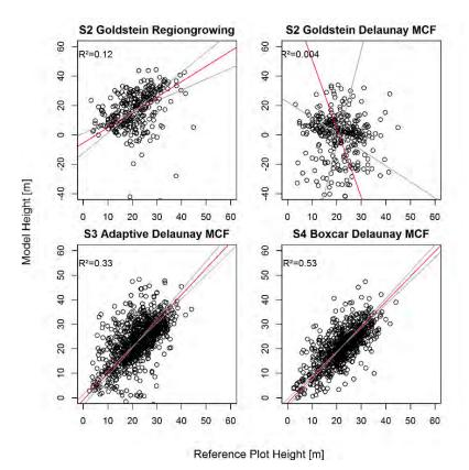
Figure 42 Reduced Major Axis Regression for different forest height models: model height (maximum model height) ~ reference plot height. Red line: Regression line, grey lines: Confidence interval around regression line visualizing 95% confidence interval of regression gradient.
