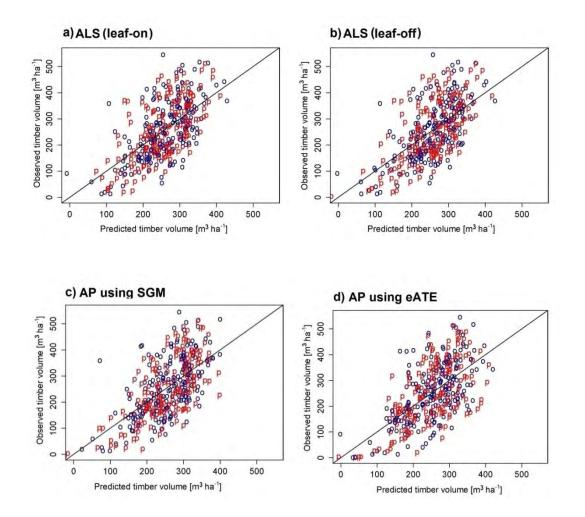
Figure 59 Predicted versus observed volume for all the four datasets based on multiple linear regression model (a) ALS (leaf-on), (b) ALS (leaf-off), (c) AP using SGM and (d) AP using eATE
