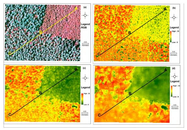
Figure 54 Final output maps of the CHMs, where the transect line was placed over (a) RGB (small subset of study area) (b) CHM<sub>ALS</sub> (c) CHM<sub>SGM</sub> and (d) CHM<sub>eATE</sub>
