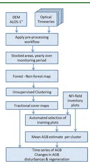
Figure 14 Workflow for estimating above ground woody biomass and stem volume based on optical time series imagery and field inventory plots.
