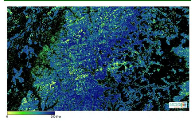
Figure 23 Above ground woody biomass estimates for the year 2002. Large areas which were damaged by the storm "Paula" in 1999 are characterised by low above ground woody biomass.
