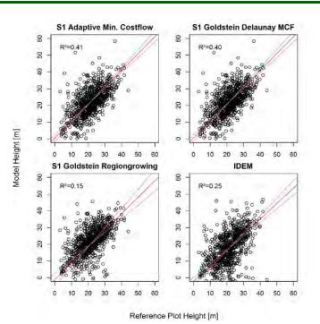
Figure 43 Reduced Major Axis Regression for different forest height models: model height (maximum model height) ~ reference plot height. Red line: Regression line, grey lines: Confidence interval around regression line visualizing 95% confidence interval of regression gradient.
