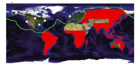
Figure 62 Restriction of forest mapping capability of BIOMASS due to Space Object Tracking Radar (ESA 2012, page 172)
