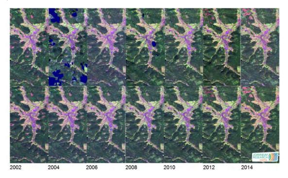
Figure 15 Result of noise-reduced and gap-filled time series (second column) compared with the input atmospherically corrected time series (first column) for a sub-region in the German demonstration site. Areas not covered by satellite measurements in the respective year are drawn in blue in first row.
