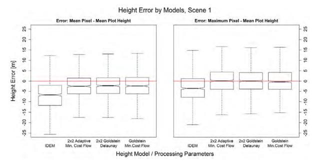
Figure 37 Scene 1 + IDEM: Height Error: mean / maximum model height – mean stand height Comparison of well performing forest height models to each other and IDEM and comparison between the use of mean- and maximum model height values with regards to the errors. Processing Parameters: Number of looks, applied noise filter and phase unwrapping of the particular forest height model used for the analysis. Red Line: Zero line.
