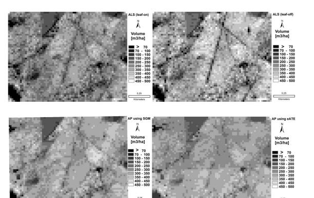
Figure 60 Timber volume prediction maps (m<sup>3</sup> ha<sup>-1</sup>) derived from (a) ALS (leaf-on), (b) ALS (leaf-off) (c) AP using SGM and (d) AP using eATE using multiple linear regression models
