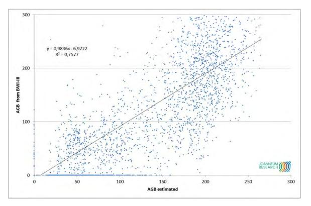
Figure 29 Independent accuracy assessment for estimation of above ground woody biomass. Scattergram and linear trendline based on n=5.167 sampling locations (each consisting of four NFI-plots) from the third national forest inventory of Germany.
