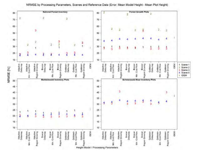
Figure 40 NRMSE of all forest height models by processing parameters, scenes and reference datasets for the mean model heights compared to the mean field heights. Height Model/ Processing Parameters: applied noise filter and phase unwrapping of the particular forest height model used for the analysis
