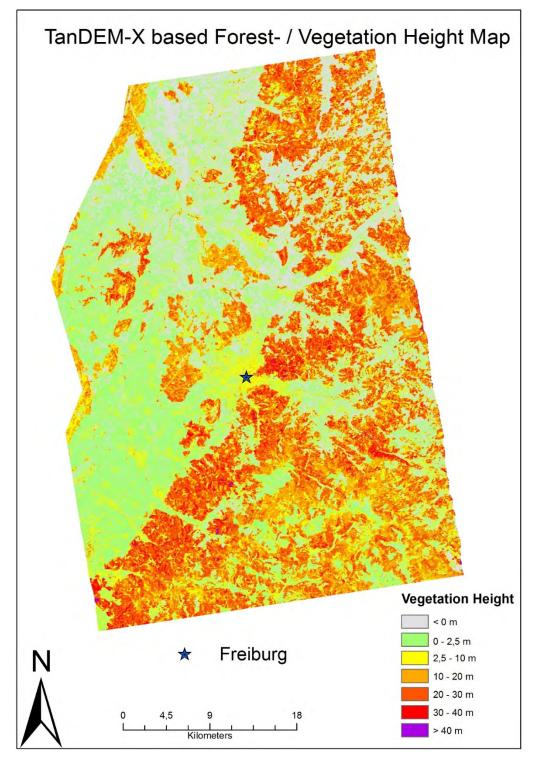
Figure 36 Forest / Vegetation Height Map, Scene 1, Adaptive Filter, Minimum Cost Flow Phase Unwrapping
