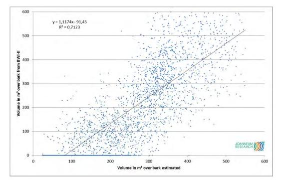
Figure 18 Stem volume - Scattergram and linear trendline for un-calibrated estimates based on n=20.688 NFI-plots
