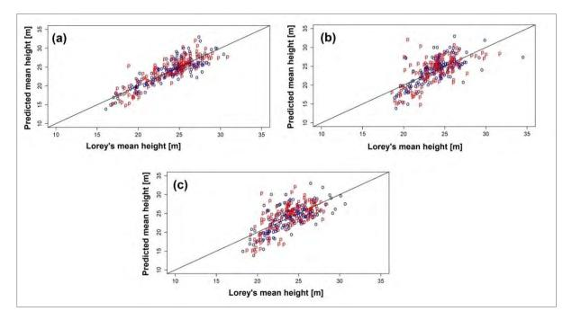
Figure 56 Lorey's mean height (LMH) (x-axis) plotted against predicted mean height (y-axis) (a) CHM<sub>eATE</sub> (b) WorldView-2 CHM and (c) TanDEM-X CHM
