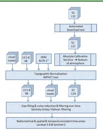
Figure 13 General pre-processing workflow, based on optical time series imagery for Landsat and Sentinel 2.
