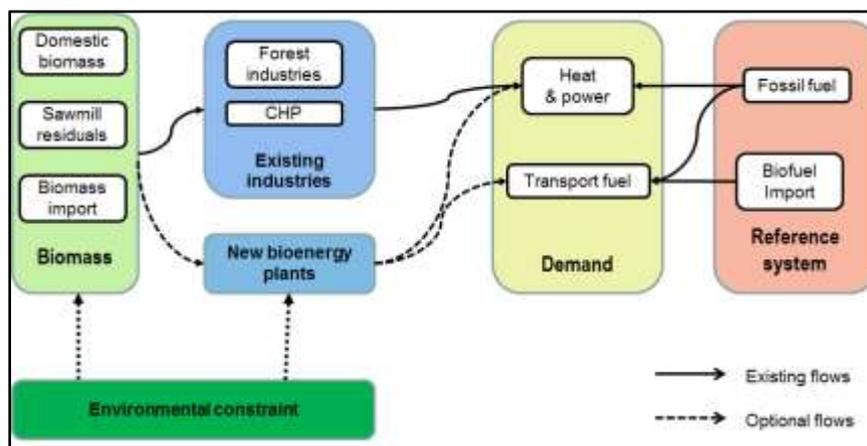
Figure 1: Overview of the full supply chain analyzed in BeWhere.
